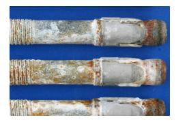
Zinc-coated carbon steel Zinc coated steel typically corrodes uniformly. Steel corrosion starts when the zinc protection is mostly consumed.
