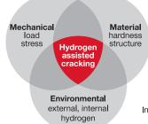
Influencing factors for hydrogen assisted cracking
