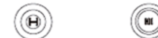
FIGURE 4—DEPICTION OF IDENTIFYING HEAD MARKINGS FOUND ON TOP OF THREADED STUDS: "H" FOUND ON CARBON STEEL STUDS AND "HI" FOUND ON STAINLESS STEEL STUDS
