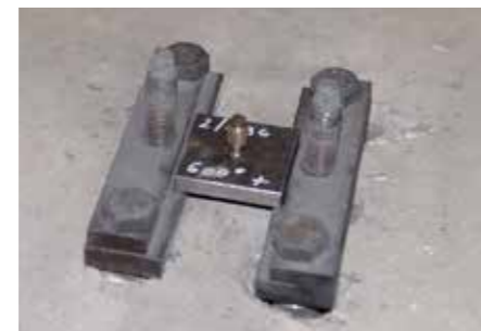
X-BT on 8.0 mm base plate
