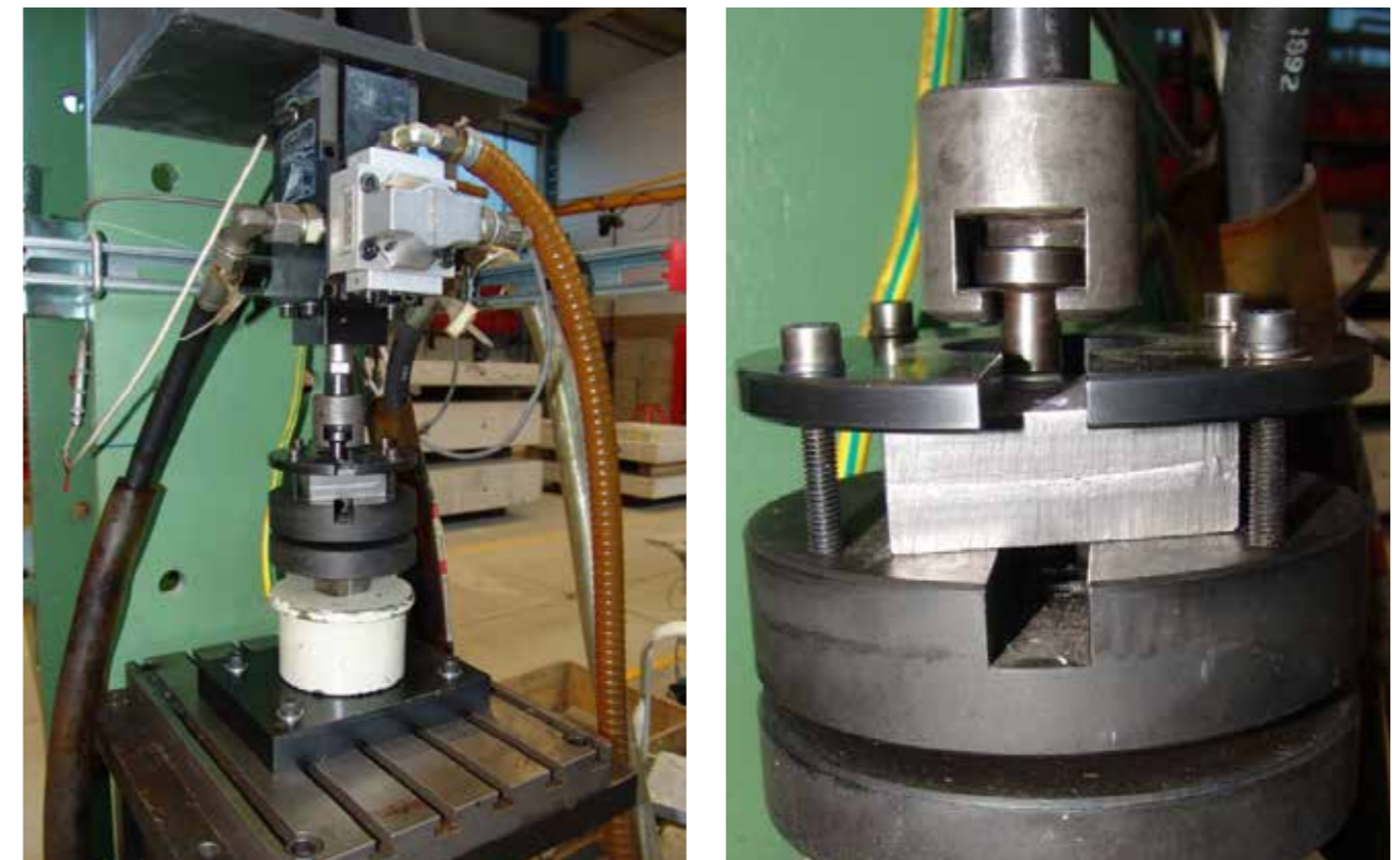
Figure 5. Servo-hydraulic test setup for tension fatigue tests
