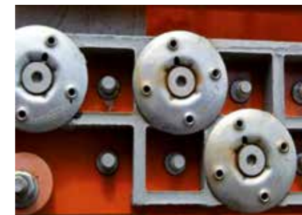
Sea water test rig with test specimens installed (X-BT with and without X-FCM grating discs).
