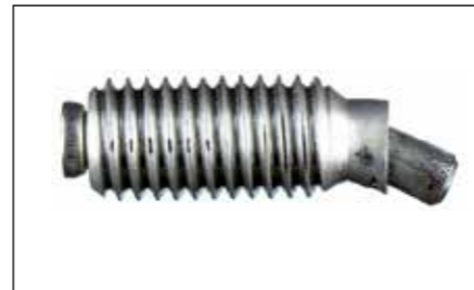
Plastic deformation of X-BT
