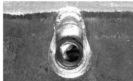
Plastic deformation of base steel
