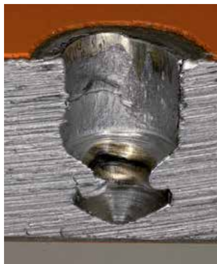
Steel base material after 7 years of exposure to sea water and pull-out of the X-BT fastener. The hole appears clean and no evidence of corrosion is visible.
